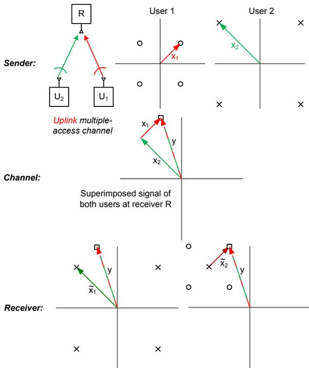
Figure 2. (Uplink) Superposition example. Here a QPSK constellation is used.
