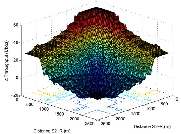
Figure 10. Throughput gain of SPCwMDPlus over 802.11 with OAR.
