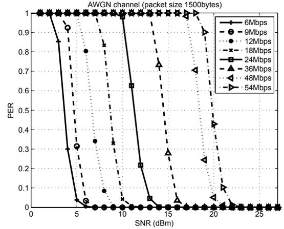
Figure 9. Packet error rate (PER) vs. SNR in an AWGN channel for large packets (1500 Bytes).
