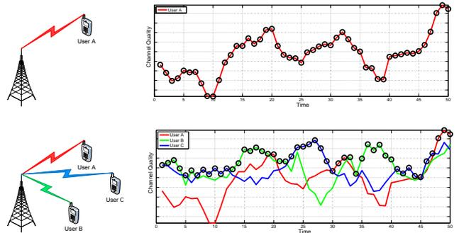
Figure 1. Wireless network with only one user (above) and multiple users (below) and a fading channel.
