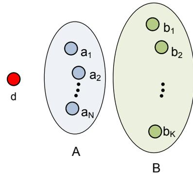
Figure 15. Network where each node from group A (B) has the same average SNR towards the gateway node  $d$ .
