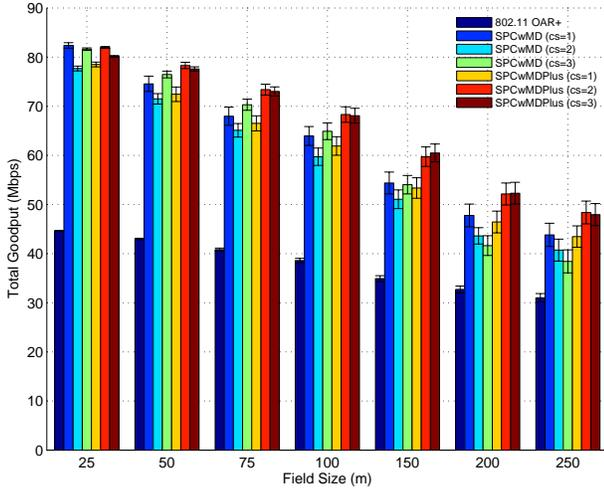
Figure 13. Average throughput ( $\pm$  standard error of the mean) for NLOS scenario.
