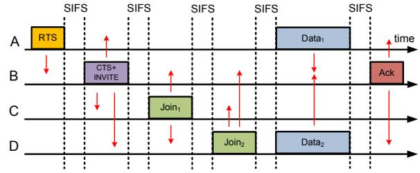
Figure 4. Illustration of the MAC operation in the basic version of SPCwMD.
