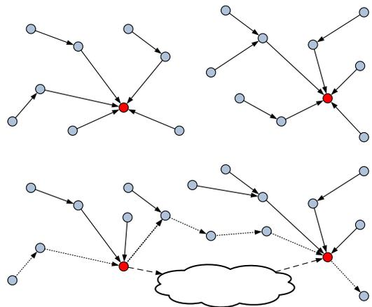
Figure 3. Wireless community mesh network with pure mesh nodes (blue) and gateway mesh nodes (red). In the first scenario (upper) gateway nodes are used to provide Internet access whereas in the second scenario (lower) the gateway nodes are connected by a backbone network (e.g. Internet) thus allowing traffic to be directed through the backbone (dashed line).
