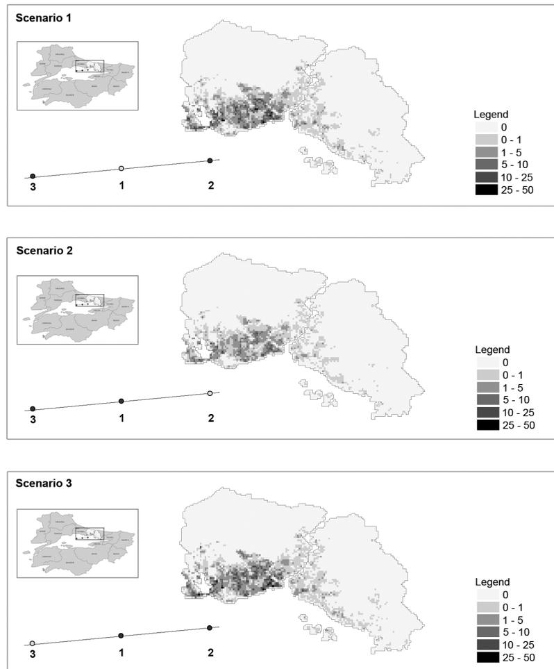
**Fig. 7.** Comparison of complete building damages of the three simulated scenarios for the 1509 earthquake.
