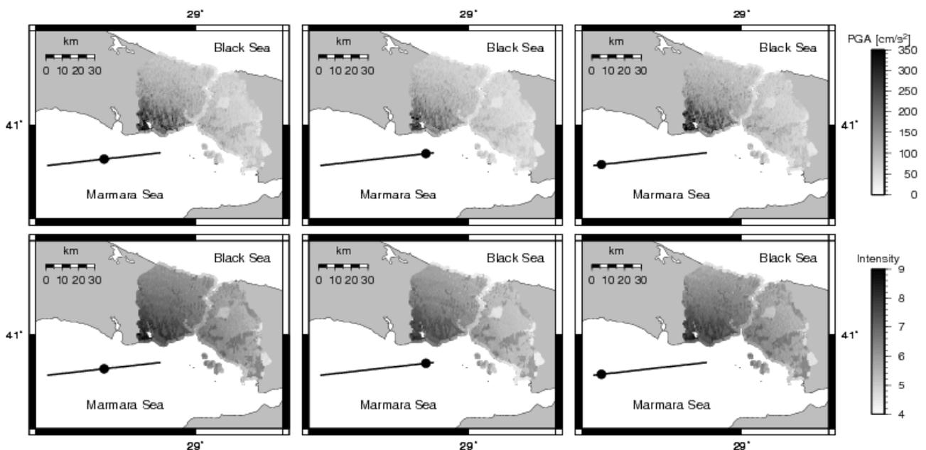
**Fig. 2.** Distribution of simulated PGA (top) and seismic intensity (bottom) of the 1509 scenario in Istanbul. The black lines represent the fault, and the solid black circles mark the location of the epicentre.
