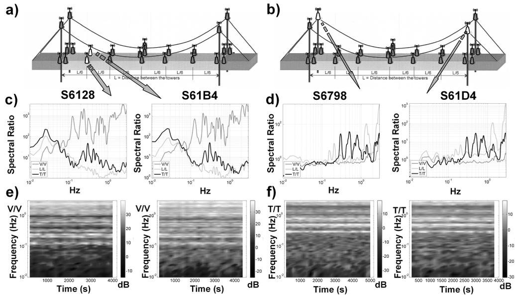
**Fig. 4.** Results for pairs of WSUs. (a) Selected sensors (*white symbols*) placed at the bridge's deck. (b) is similar to (a), but of sensors placed on top of the bridge's towers. (c) and (d): Spectral Ratio (SR) functions for the vertical (*dark gray*), longitudinal (*light gray*), and transversal (*black*) components of motion. (e) and (f)
