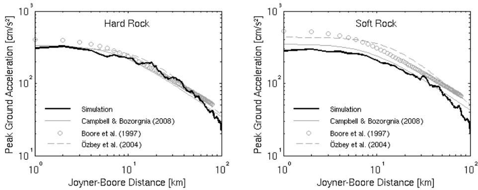
**Fig. 1.** Attenuation of PGA with distance from the earthquake for hard (left) and soft rock sites (right) of the 1509 scenario, with the hypocentre located in the middle of the fault. The simulation curves are smoothed over 5 km.
