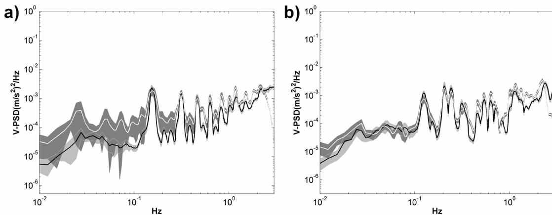
**Fig. 3.** PSD functions for the vertical components of motion. Average PSD plus  $\pm 95\%$  confidence interval for SOSEWIN (white and dark grey, respectively) and Guralp (black and light grey, respectively). (a) Sensors located on the middle of the bridge's deck (i.e. WSUs over the deck, and Guralp within the deck). (b) Similar to (a), but with nodes located at about 1/3 of the way along the bridge's deck.
