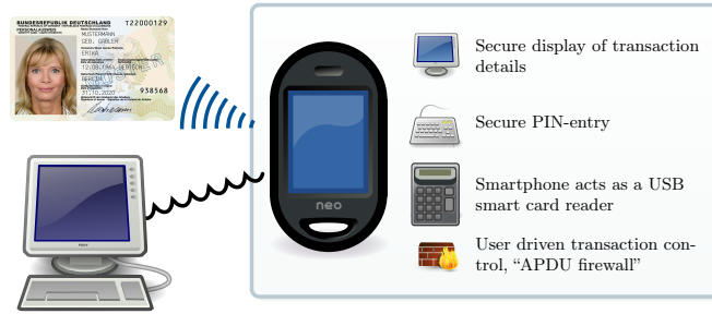
Fig. 1. Using the mobile smart card reader as secure input and output device for a computer that may not be trustworthy
