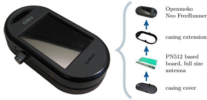
Fig. 3. Openmoko mobile phone with casing extension, PN512 board and antenna.
